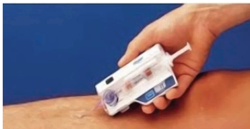
(Top) Above knee cadaver used in lab studies to create a model of lower leg compartment syndrome. (Bottom) Demonstration of the Intra-Compartmental Pressure Monitor.
